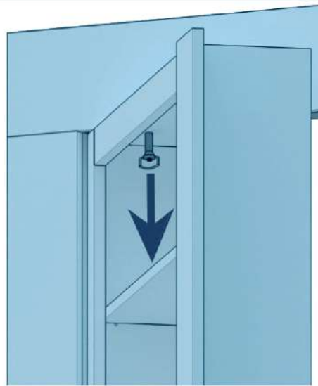
2. Detach Bookcase from Bookshelf Door Frame by removing Rotating Pin. You will need to push the Pin Button and pull the Pin out to remove it.
