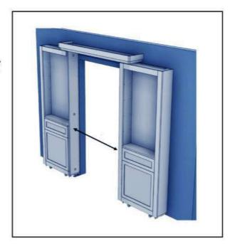
Connect the top rail of the crown molding to the rail on the uppercase.
