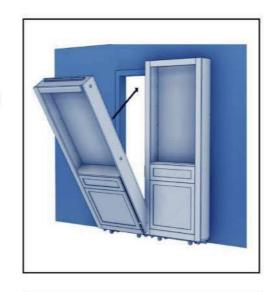
When lifting the bookcase up against the wall, place the bottom rail in the roller guide.
